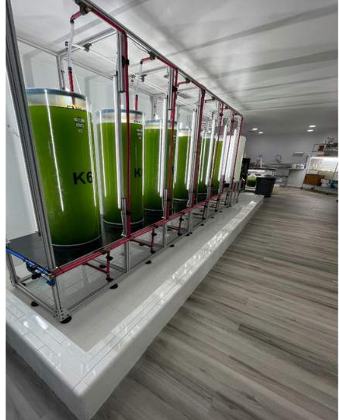
Algae are grown in translucent tanks with LED grow lights. Photosynthesis draws down carbon and releases oxygen, the only byproduct of production.
